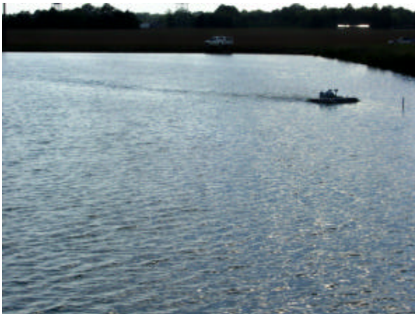
The RELIANT Model WQA showing bubble stream and flow pattern during Stage 1. Only 1.5HP can move all the water in an 8 acre pond.
